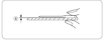
To check needle straightness, place the flat side of the needle onto something flat (a needle plate, glass etc.) The gap between the needle and the flat surface should be consistent.
