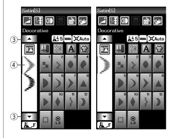
To delete a pattern in the middle of a combination, press the cursor key to select the pattern you wish to delete. The stitch image of the selected pattern turns red. Press the delete key to delete the selected pattern.
